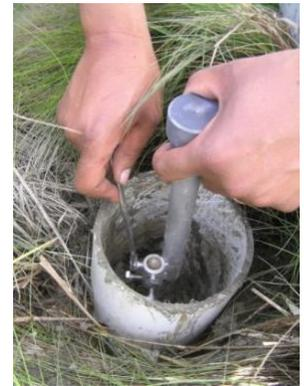
13. Overfill the PVC pipe, smoothing the top so that it sheds water.
