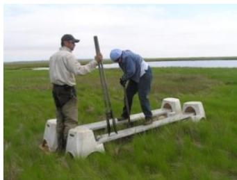
5. Place the driving tip on the first steel rod and counter tighten with 2 vise-grip pliers.
