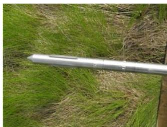
6. Drive the first stainless steel rod into the marsh by hand, keeping it as vertical as possible. Use 2 observers to indicate rod is plumb.
