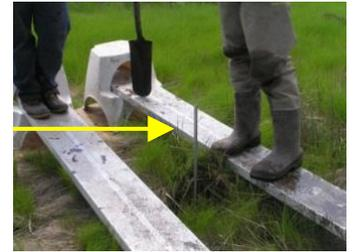
7. Connect successive rods, flipping each new rod so that a new screw is on top. Hand screw in the driver head. Next ensure the new rod is tightened into the one below using 2 counter-turning vise grips. Remove the lower vise grip and turn the entire assembly, tightening all the rods into one unit.
