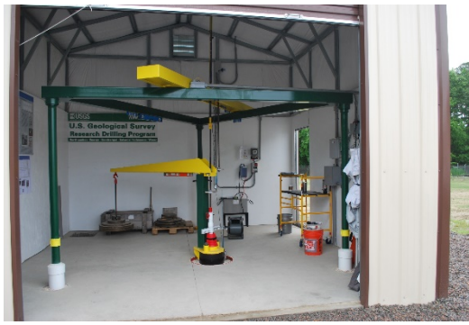
USGS geologists will analyze data produced by an extensometer installed at the SWIFT Research Center to determine changes in land subsidence.
